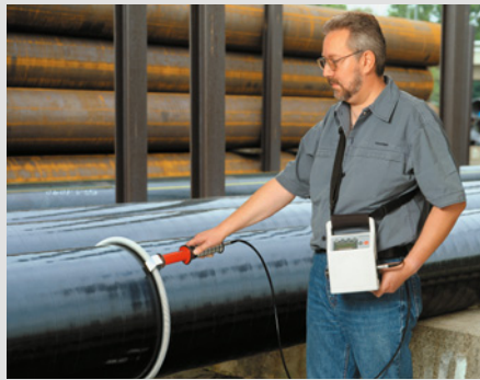
Porosity detection on pipelines
